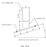
C. Rafter bracket as manufacture by "Beam Lift" or approved equal.
