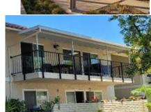
2.9 Patio & Balcony Awnings: An architectural projection located at ground or balcony levels that provides partial weather protection but remains open on three sides. The entire awning system is attached to and wholly supported by the building structure. It can be fixed or fully retractable.
