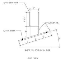
C. Rafter bracket as manufacture by "Beam Lift" or approved equal. EXCEPTION - Building guttering may be modified to 5 inches wide to accommodate rafter bracket installation
